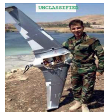
One of the UAVs used to attack Russian bases in Syria on 5-6 January is displayed upside-down to show its IEDs mounted on rails.
